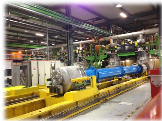
Part of the magnetic testing laboratory which checks the magnet used to focus the beam of particles in the LHC
